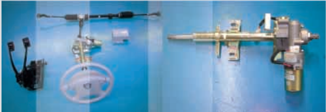
福林生產的電動助力轉向器 Electric Power Steering made by Fulin
