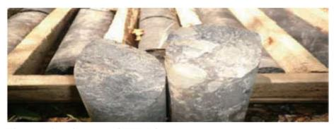
Figure 5-6: Drill cores of ZKD1 from Dumuheshangtou Property
